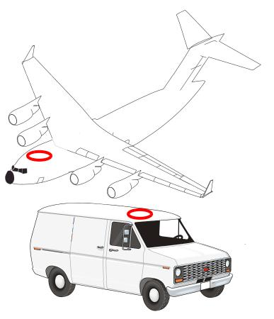
The graphic above shows examples of where the ANT-A72GLA-TW-N or ANT-A72GLA4-TW-N antenna may be located on an aircraft or vehicle (not to scale).
