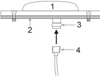
6. Attach the other end of the coaxial cable to the antenna input port of the receiving device. The receiving device must be able to provide power as detailed in the SPECIFICATIONS section of this guide. All NovAtel GPS receivers provide the necessary power through their antenna RF connectors.
